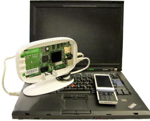
Figure 3. Our setup: A computer to monitor traffic and perform attacks, a victim phone and an SFR femtocell.
